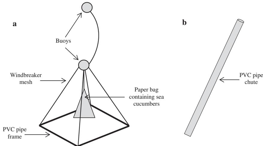
Fig. 2. Trial methods equipment design diagrams (a) temporary cage and (b) chute.
